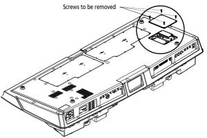
When turning the unit upside-down, get a bunch of newspapers or magazines and place them under the four corners. Always orient the E-80 in such a way that no buttons or controls get damaged. When turning the E-80 upside-down, handle with care to avoid dropping it or allowing it to fall or tip over.
